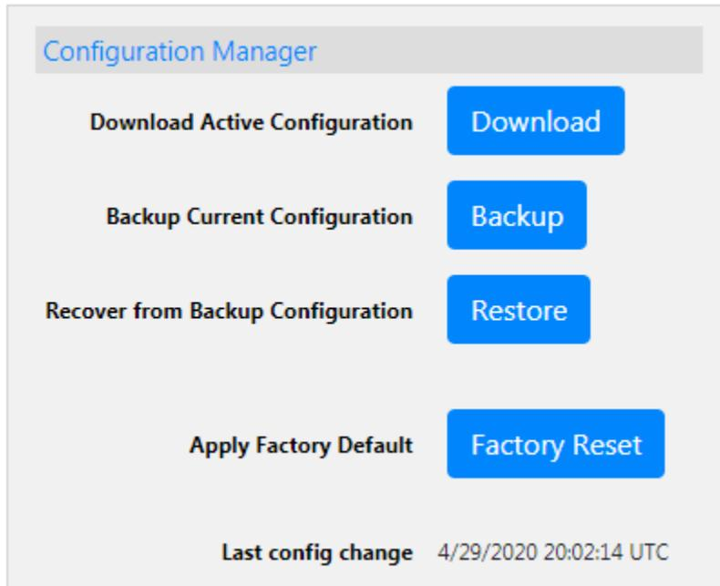
**Download Active Configuration:** This option is used to provide your support team the active S400 PRO configuration. Click on this button and send the resulting configuration file to your support contact.
