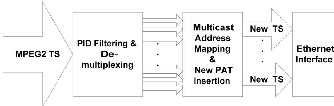
**Figure 1 – Novra Receiver Enhanced Capability**
